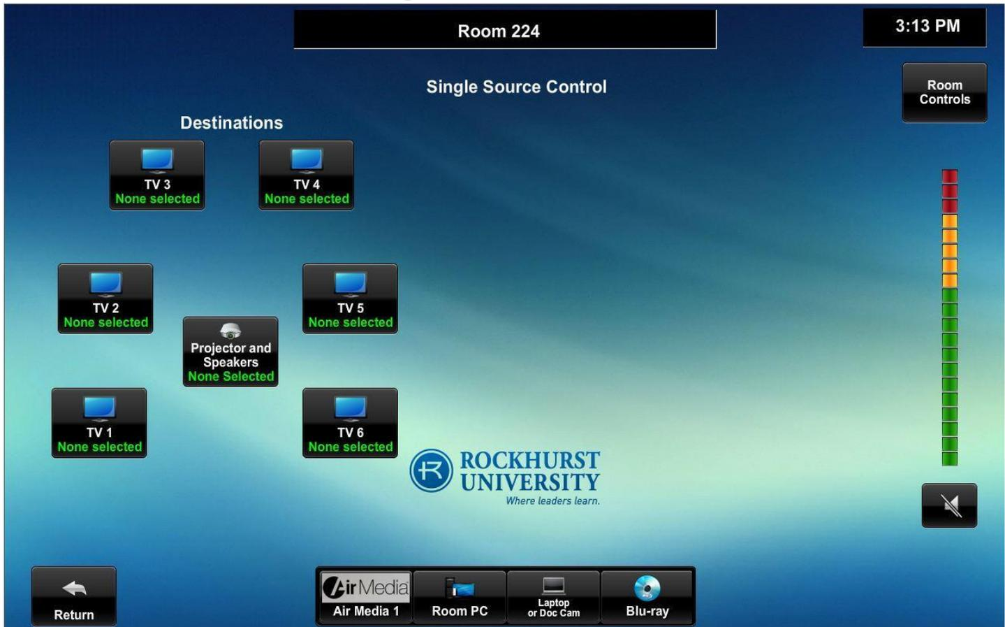
Single Source Mode is hard coded to allow you to select a source (centered on the bottom of the screen) and it will display to all of the “Destinations”. In this mode you are limited to a single AirMedia device that can be displayed
