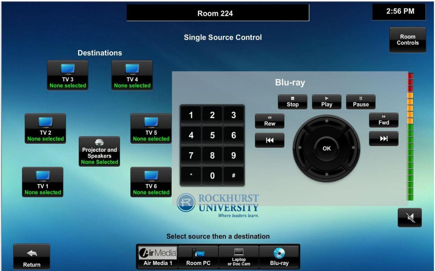
When Blu-ray is selected as a source the controls will pop up on the right hand side of the screen. Included are the basic Play controls the directional pad for navigating menus as well as the number pad
