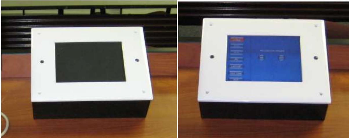
Now you should have a display with options running down the LEFT side; these buttons are called “source switches”, which allow you to choose the desired equipment. If there are buttons on the right, that is fine for now. It just means a source has already been selected. A selection is denoted by a red button, as you will see in the next few pictures.
