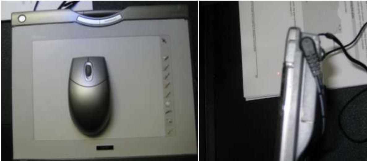
**LAPTOP** The laptop button has the same limited controls as the PC, but will take less time for the initial command to execute. The cables for connecting a laptop are located on the top of the station. If the station does not project your laptop monitor image, you will need to activate the external monitor connection on your laptop (the Fn + F8 keys on most Dell laptops).
